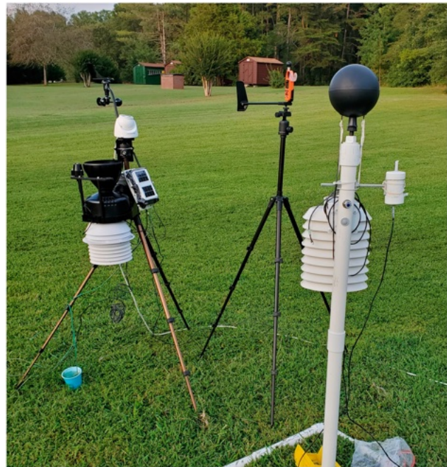
FIG. 3. Field work instruments (WBGT meters and weather station). The WBGT meter is on the right, with a black globe thermometer, a natural wet-bulb temperature probe situated in a water reservoir, and a dry-bulb sensor in a radiation shield. A weather station (on the left) and a Kestrel 5400 (in the center) were also collocated with the WBGT meter.
