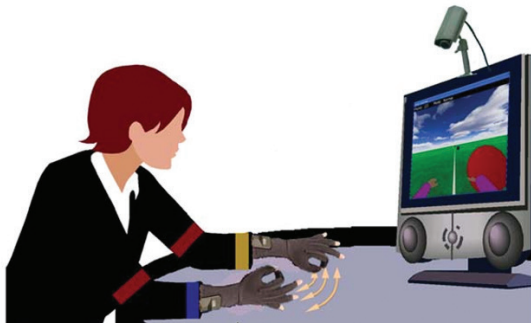
Fig. 2. [5] The Rehabilitation Gaming System is depicted above. Data gloves detect movement from the user and map them in real-time to the virtual arms on the display. The PTM (Personalized Training Module) measures the number of successful events completed by the user and adapts the difficulty for the next trial.
